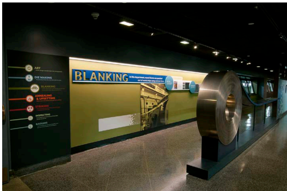
Explaining how coin blanks are created from huge rolls of metal strip purchased by the United States Philadelphia Mint.
