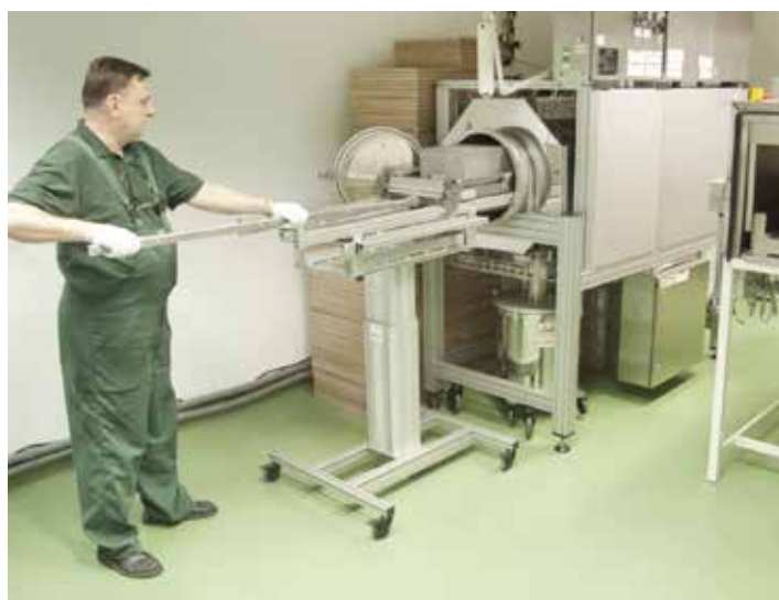
Loading the coins into Beneq equipment for ALD process.
