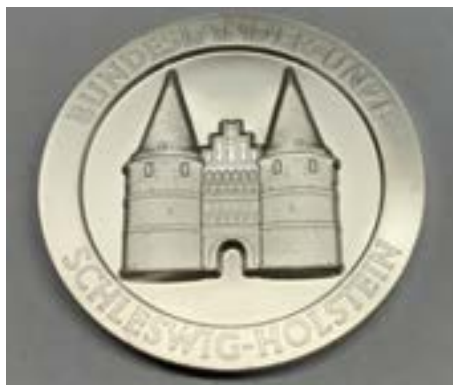
High relief coins struck from a regular blank and a powderBLANK applying a minting force of 80 tons.
