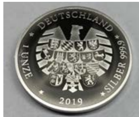
High relief coins struck from a regular blank and a powderBLANK applying a minting force of 80 tons.
